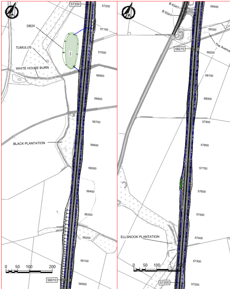
Figure 4-3 - Highway Drainage Layout and Detention Basin DB24
