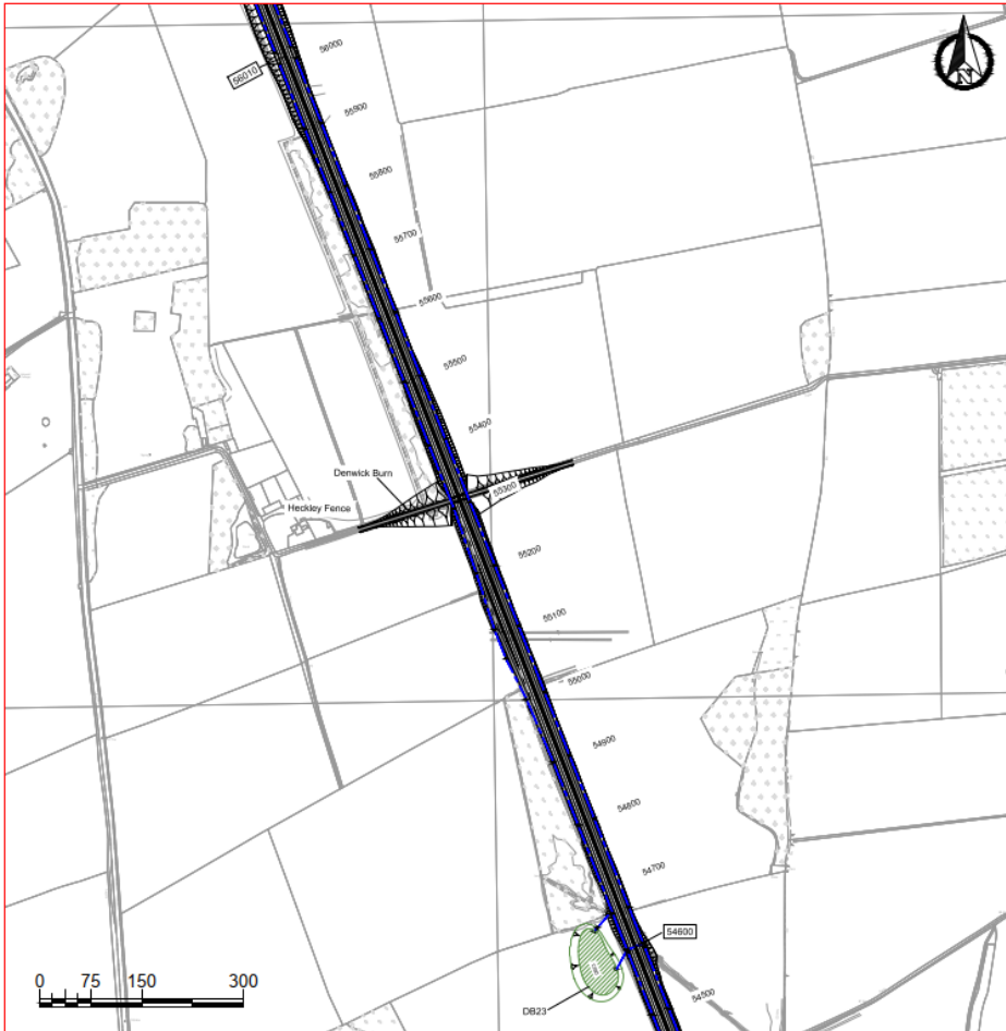
Figure 4-2 - Highway Drainage Layout and Detention Basin DB23
